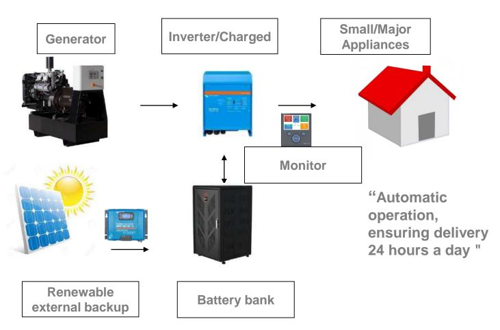
In a very reduce space the equipment integrates all the components necessary to supply electricity, engine, alternator, inverter/charger, battery bank grid, electronic devise for managing the equipment and connection box for external rolling support. Furthermore, it is soundproof and insulated to avoid noise, easily installed and carried on remote areas.
